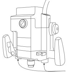
For maximum performance and smoothest plunging action all plunge posts require a light film of lubrication. We only recommend using STP® MOTOR OIL TREATMENT.
